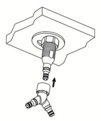
• For connectors with washers, put washer inside, thread and tighten quick connect adaptor to spout shank then insert Y connector into the end of quick connect adapter on the inlet end of the spout shank. Push until a "click" sound is heard. Pull down the Y connector to test engagement.
