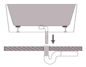
• Connect the drain pipe to the bathtub drain using the provided parts. Ensure the connections are tight and secure. Use a Ptrap and tubing cutter to connect the drain to the existing plumbing.
