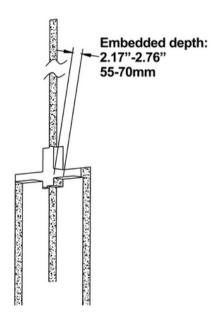
2. Install main body and inlet pipe.
