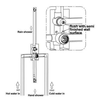
3. Make sure the inlet pipe surface slightly below the tile surface/finished wall surface.
