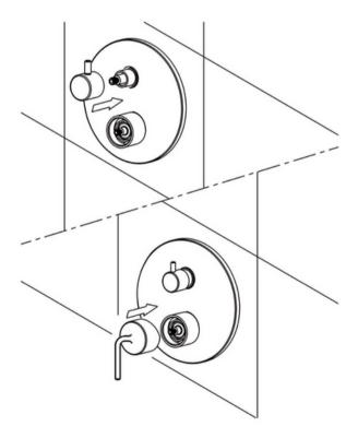
6. Mount Holder for top sprayer, outlet for top sprayer, and holder for hand held sprayer. Wind teflon tape around screw.
